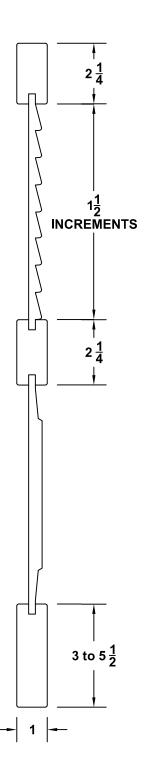
Millennium Wood Composite Combination shutters have eased edge stiles and rails. They are built using dowel construction, raised panels (raised 1 side) and "flush face" design (all stiles and rails are the same thickness). Faux louvers are used on this combination shutter. Millennium shutters are primed with an option for prefinishing with either standard or custom colors.
